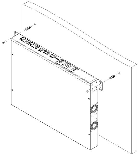
Figure 4-4. Installing the Switch on a Wall
